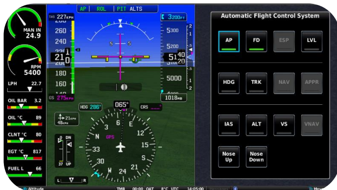
Autopilot display: AP mode and default ROL and PIT engaged. Servomotors drive the flight controls to follow FD commands.
