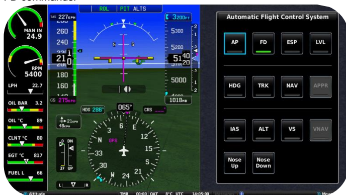
Autopilot display: FD mode and default ROL and PIT engaged Servomotors do not drive flight controls.
