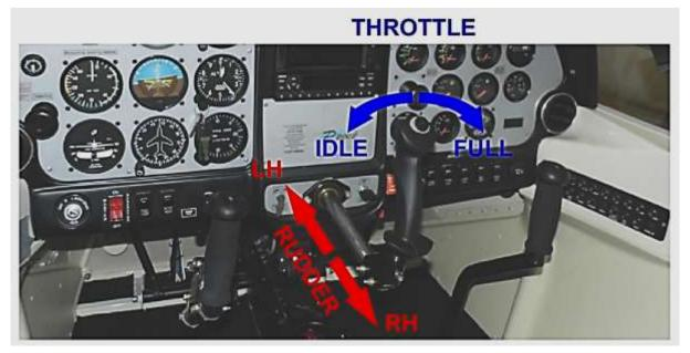
Fig.A14-7. Hand controls schematic
