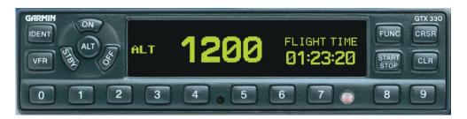
Figure 1 – GARMIN GTX330 Transponder
